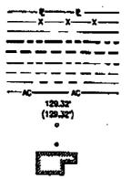
PROPERTY (DEED) LIME FENCE LINE CENTERLINE PROPOSED RIGHT-OF-WAY LINE PROPOSED EASEMENT LINE DOSTING RICHT-OF-WAY LINE EXISTING EASEMENT LINE LAND SECTION LINE ACCESS CONTROL LINE MEASURED DATA RECORDED DATA SET FROM PIPE WITH RED CAP STAMPED W/STHA ROW FOUND MONUMENT EXISTING BUILDING
